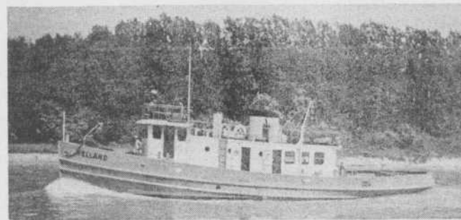
The photos show the new tug "Welland" which was built to replace an old steam-driven tug mainly for towing various items of Welland Canal floating plant, such as the gatelifter and derrick scow.
