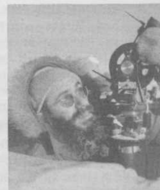
Radio provides the year round link with the outside world as well as sending out weather data at station intervals. (R) Steve Kolin, from North Battleford, Sask., at Isachsen using a theodolite - a telescopic device used to follow the course of the pibal balloon.
