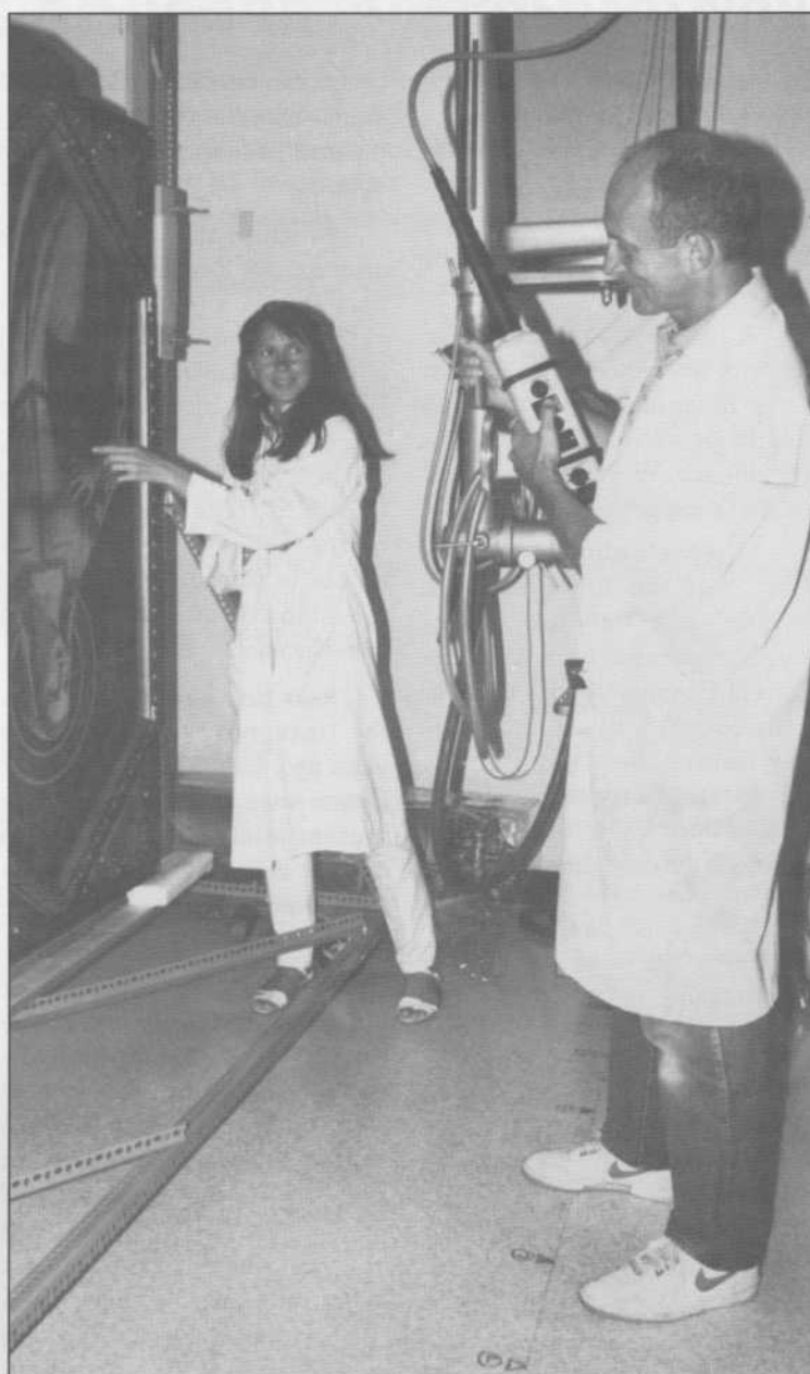
CCI Conservator Helen McKay (left) sets up an X-ray of La Peinture Mystique with recording and documentation technologist Jeremy Powell to obtain sub-surface details as part of CCI's examination of the work.
