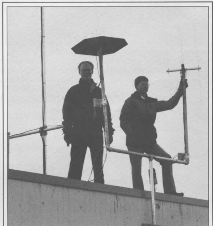
Tests of the IRMA (Integrated Remote Monitoring Apparatus) system are occurring in regions across the country. Here, Wayne Janzen and Dave Taschuk check the system's UHF and VHF direction-finding antennas for a test at the Edmonton District Office. See "Regions and Headquarters co-operate on IRMA tests" on page 5.
